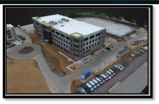
Building Information Modeling - Using ground control points, our drones can survey and develop asbuilt site data accurate to within 1/4".
